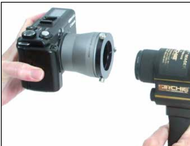
FIGURE 9 —Slide the Camera Coupler over the eyepiece of the Imager.
