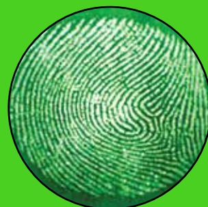
CYANOACRYLATE FUMED fingerprint on soda can photographed with a digital camera connected to the KRIMESITE™ IMAGER .
