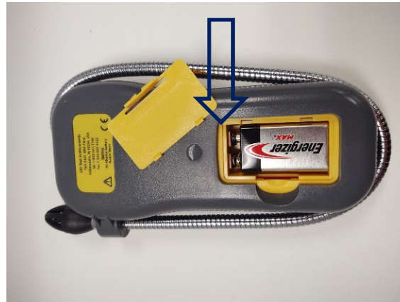
Plug-in the 9v battery
