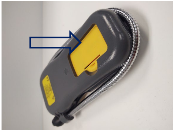
Remove battery cover (back side of instrument)
