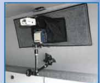
Upper compartment windows provide an excellent location for auxiliary cameras or directional microwave antennas.
