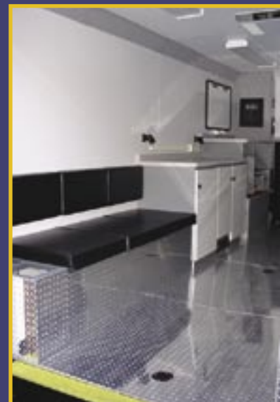
"V" shaped, sloped, bright aluminum diamond plate flooring channels water to floor drains.
