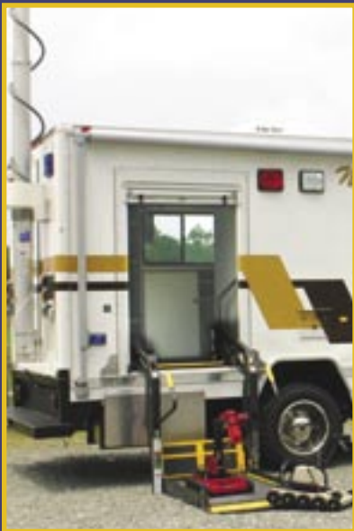
Available roll-up side access door with hydraulic lift allows for quick and easy Bomb Robot deployment.
