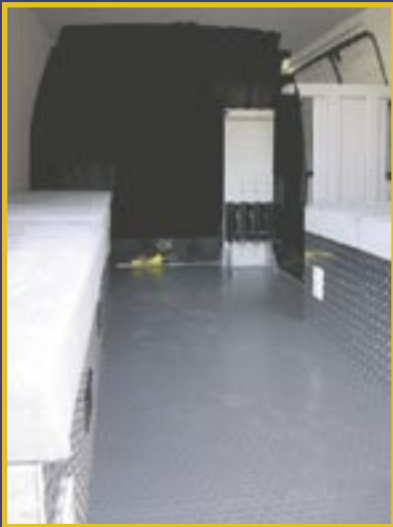
Bench seating, rubberized no-slip flooring, secure weapon locks and tactical red/white lighting.
