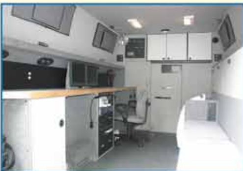
Open countertop design allows space for equipment such as a briefcase-style body wire gear, microwave video receivers and telemetry control equipment.
