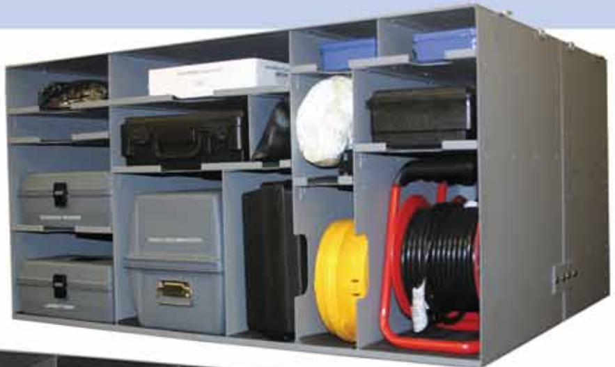
Pictured Above: Module Accessible From Rear Hatch
