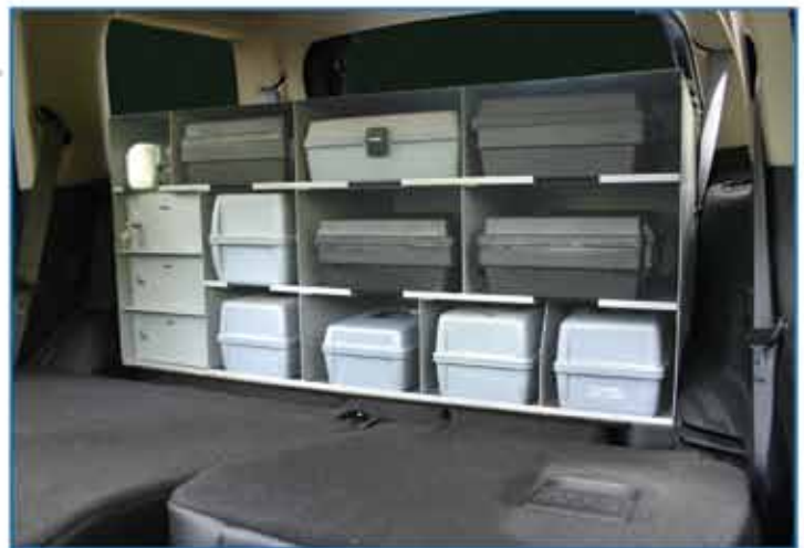
Fully functional second row seating folds downward to reveal kits on the cabinet modules second side. In an upright position, the seating secures and conceals all kits and evidence compartments.
