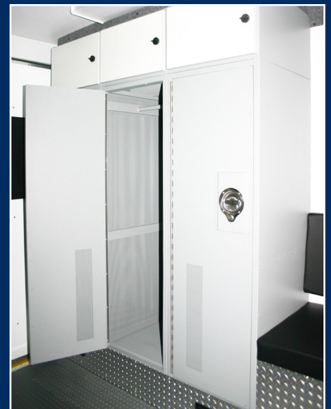
Ventilated Wet Suit Storage Locker
