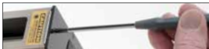
Remove the set screws from the top and bottom of the unit with a Phillips Screwdriver.
