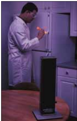
FIGURE 1 —Technician uses the UV9600 to illuminate dusted latent fingerprints.
