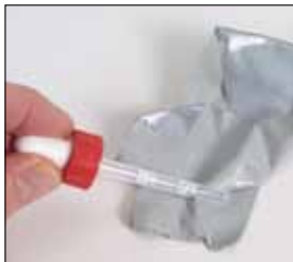
TRA20 release agent is applied to adhesive side of tape.
