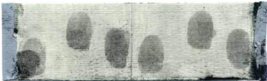
After applying TRA20 to duct tape, latent prints are revealed when processed with ASD7D Dark Adhesive Side Powder.
