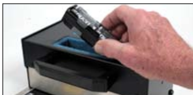
Observe the correct polarity of the batteries and re-install the magazine into the battery compartment.
