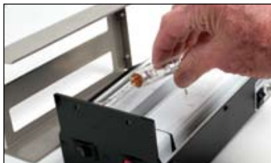
Grasp the old lamp between the thumb and forefinger, twisting it 90-degrees to remove it from the sockets.
