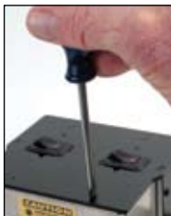
Remove top and bottom set screws to remove shield.
