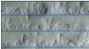
Oblique white light used with a DSLR with macro lens for close-up photos of indented writing (camera not included).
