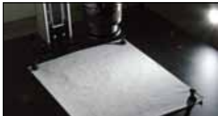
Oblique white light used with a DSLR with macro lens for close-up photos of indented writing (camera not included).
