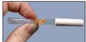
Break the ampoule between your thumb and forefinger.
