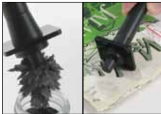
125MBA Magnetic Burnishing Applicator (left) and its use with lifting material (right).
