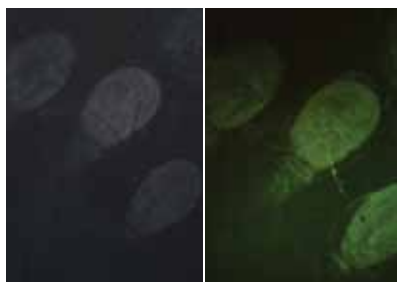
505nm —The left photograph shows prints developed on a black background using cyanoacrylate fuming and enhanced with Rhodamine 6G. This solution fluoresces well with the higher 505nm Light as shown right. (Orange barrier filter used for photograph.)
