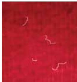
590nm —This single dark blue fiber was located on a black shirt using the 590nm Light. The fiber is not fluorescent, but the background does show slight fluorescence making the fiber stand out against the background as shown right. (Orange barrier filter used for photograph.)
