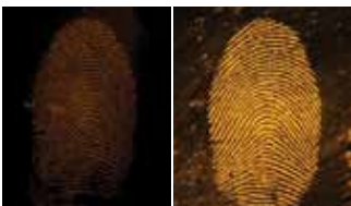
470nm —In the above prints, the left photo is a latent print on a black surface enhanced with orange fluorescent powder (no ALS). The print pops when illuminated with the 470nm (right). (Orange barrier filter used for photograph.)
