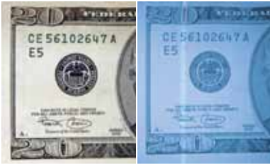
395nm —In an effort to thwart counterfeiting of US currency, a fluorescent stripe (with printing on it) is embedded between the layers of paper. In the left photo, this stripe is not visible to the naked eye or at any light frequency other than ultraviolet. The right photo was taken when the money was illuminated with the 395nm UV Light.
