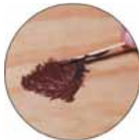
FIGURE 3—Apply the material to the surface to be cast.
