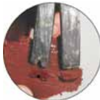
FIGURE 4—After peeling the cast away from the surface, compare it with the suspect tool.
