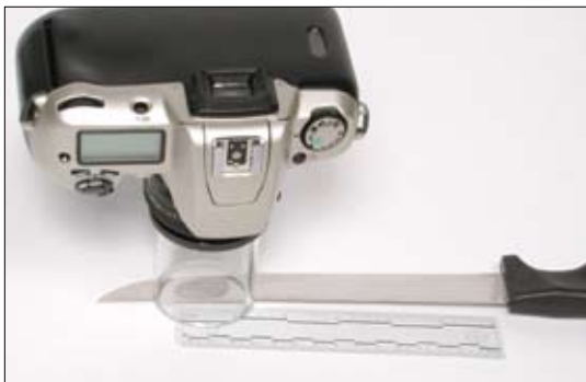
FIGURE 4 —No. EVD52 Lens Adapter attached to camera is used to facilitate a photograph of a developed latent fingerprint on the knife blade. The resultant print is shown to the right at actual size.
