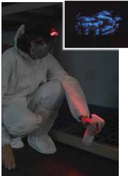
The area to be searched and treated with Luminol is illuminated by the RED light of the LumaVision™. The inset is the resultant bloody footprint found.
