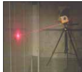
FIGURE 11 —Introduce Photo Laser Smoke (LTF100S) into the scene to make laser beam visible for photos.
