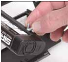
Unscrew the wing nuts securing the lights to the support rods and remove.
