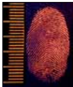
DFO processed latent print @ 505nm, viewed with orange barrier filter.
