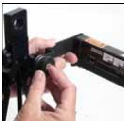
Remove the threaded knobs from the rigid support arms.
