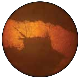
DFO enhanced prints, like the palm print shown here, are highly luminescent when viewed with the BMV100 in the blue light mode.
