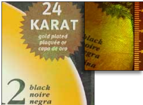
Pen box (above) dusted with LL703. Inset (top right) photographed with BLUEMAXX™ illumination.
