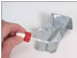
No. TRA20 allows separation of the adhesive surfaces without destroying latent prints that may be present.
